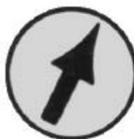
The course selector knob is used to adjust the autopilot course selector arrow to the desired course. Selection of the autopilot course automatically sets the internal VOR resolver to the identical VOR radial. Readout of VOR left-right information is made by observing the center segment of the course arrow.
