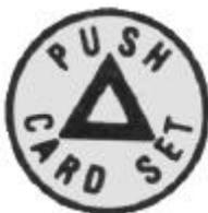
The heading selector/card set is used to move the heading bug relative to the heading card. It is also used to set the heading card to the aircraft heading by pushing in and rotating card. When setting has been accomplished the knob is released. The heading selector should not be pushed in when setting the heading bug.
