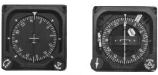
In systems equipped with an NSD-360A or other HSI, a selected intercept angle function is available while operating in the NAV, APR and REV modes.
